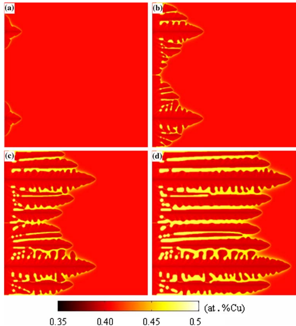
Fig. 3 Evolution process of directional solidification with the left boundary heat flux equal to 90 \text{ W/cm}^2 . a t = 0.2046 \text{ ms} , b t = 0.6820 \text{ ms} , c t = 1.3640 \text{ ms} , and d t = 2.3188 \text{ ms}
